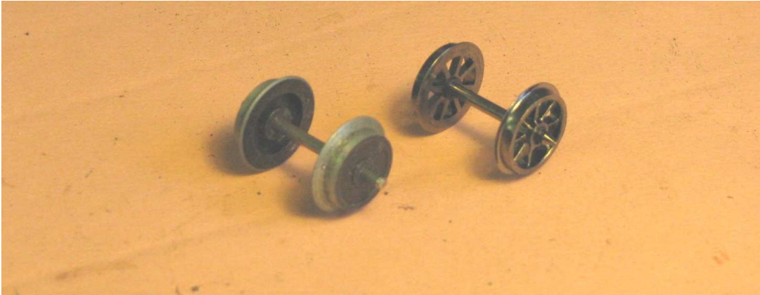
3-rail wheels (on left) and 2-rail wheels (on right). The 2-rail wheels have tiny insulating bushes between the axles and wheels.
