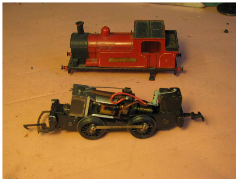
Simple Tri-ang model, showing wire bringing power to the motor from the pickups on the insulated wheels.
